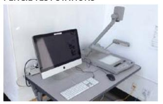
Used for quick testing of pencil drawn animation, pencil test stations utilize Mac computers running TVPaint software, capturing still images from standard-definition video downshooters. Some stations also feature large-format flatbed scanners and VueScan software. The pencil test stations are connected to the School of Film/Video file servers, so students' work can be saved and loaded to each student's folder, or uploaded to Faculty folders for submitting homework.
