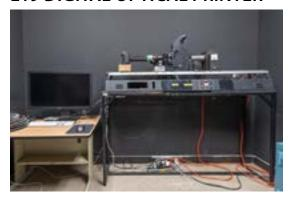
Students can learn how to be proficient with handmade filmmaking in this workspace that houses a JK digital optical printer. The JK optical printer is fitted with a digital camera, controlled with Dragon Frame software for transfer of 16mm and 35mm film to digital format up to 4K resolution. Additional facilities include a workbench and splicer for making handmade films.
