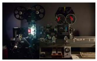
This room houses an Acme optical printer that is computer controlled and used for manipulating and re-filming 16mm and 35mm motion picture film. Additional facilities include a workbench, moviscope, splicer and air compressor.
