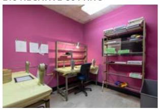
This negative cutting room houses two workbenches with rewinds for A/B rolling and cement splicing.
