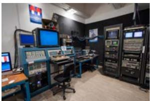
C105C Videographics is a dedicated live analog video generation and manipulation facility. Using any or all of the various generators, unique and subtle electronic images can be created. Audio sources can be used to influence the images via a Eurorack modular video synthesizer. Pre-recorded and live sources can be combined and altered with immediate results, no rendering needed. Sources for pre-recorded materials can include DVDs, DV
