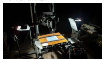
Designed for single-frame shooting, a 16mm camera body is mounted on an Oxberry stand which enables the camera to be moved towards and away from the artwork. Artwork is supported on the stand with pin registration allowing for accurate moves.
