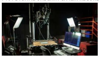
Designed for single-frame shooting, the camera is mounted on an Oxberry downshooter stand, which enables the mounted camera to be moved towards and away from the artwork. Artwork is supported on the stand with peg registration allowing for cell replacement without jumping.
